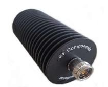
DC-4 GHz, 6 - 60 dB, 100 Watts, 4.3-10 Male to Female, Bi-Directional Operation
